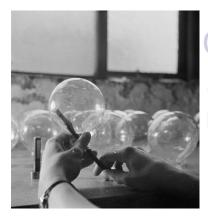
Here, a 'sticky bomb' is being examined to check the depth of the neck. It was important to know how deep the bomb was, so it could be filled with the right amount of explosive! Would you have wanted to have done this job?
