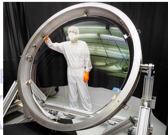
Figure 11, The large lens of the Vera C, Rubin observatory camera. The lens measures 1.57 m, making it the largest optical lens in the world
