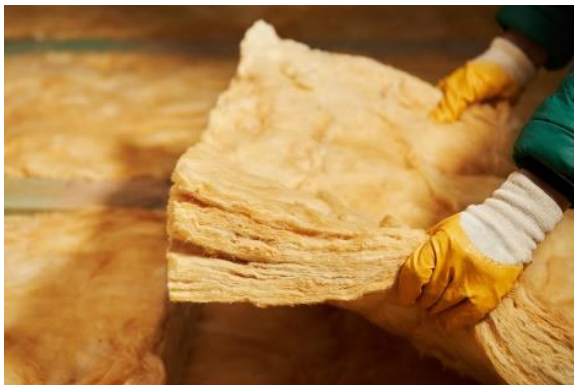
Figure 7, Fibre glass insulation
