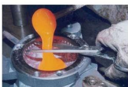
Dropping and cutting of a gather of hot glass into mould.
